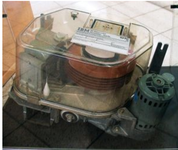
Disc dur IBM (model 62PC, "Piccolo"), de 64.5 MB, fabricat el 1979
