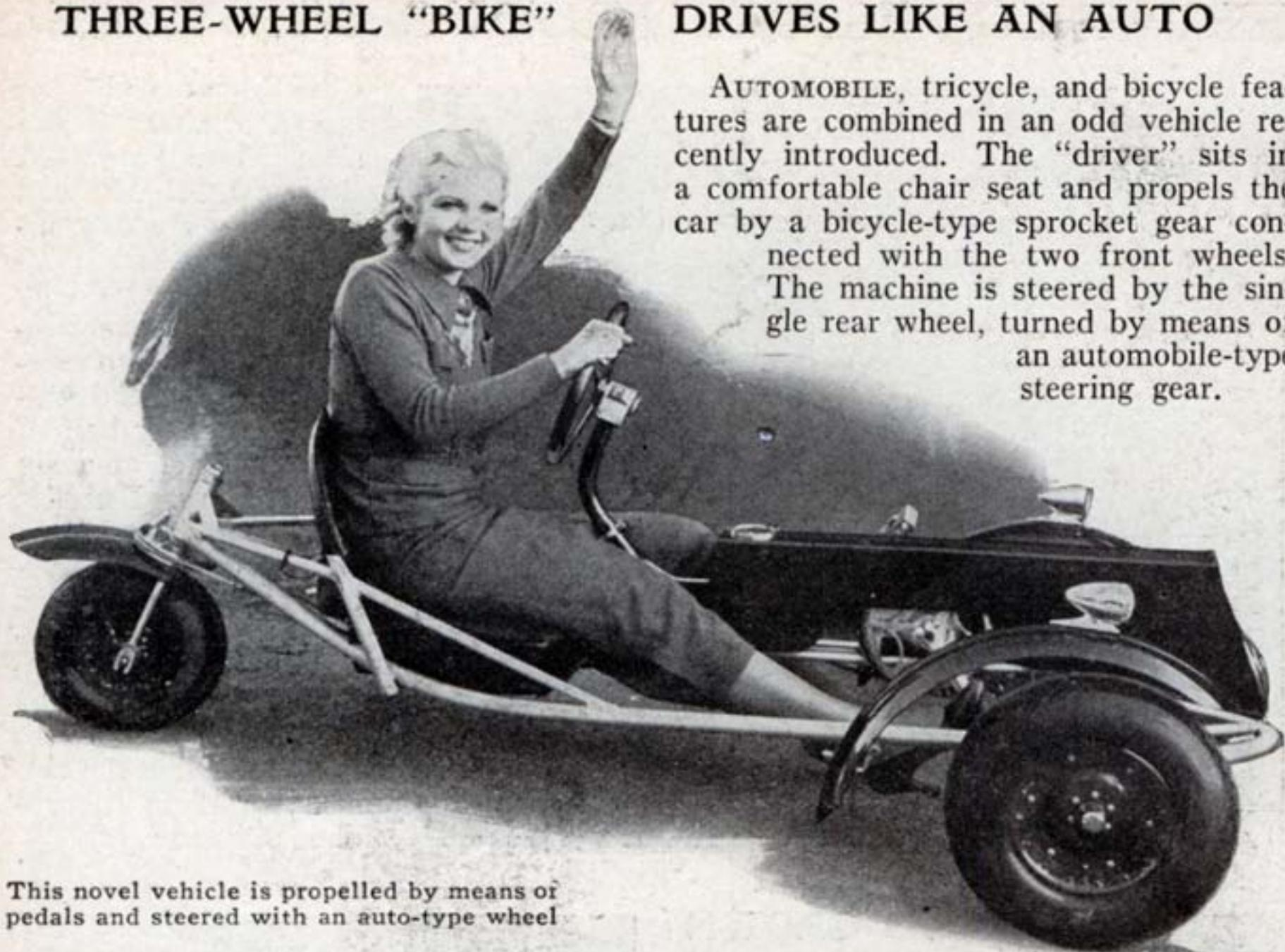
This novel vehicle is propelled by means of pedals and steered with an auto-type wheel
